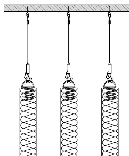
Above: Baffle with #ICS internal channel screw fixed to suspended frame such as Rondo Donn® grid or furring channel. ECD external channel may also be used fixed to suspended grid.
