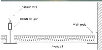
Detail: Avant 15 ceiling tiles suspended on Rondo Donn DX Grid
